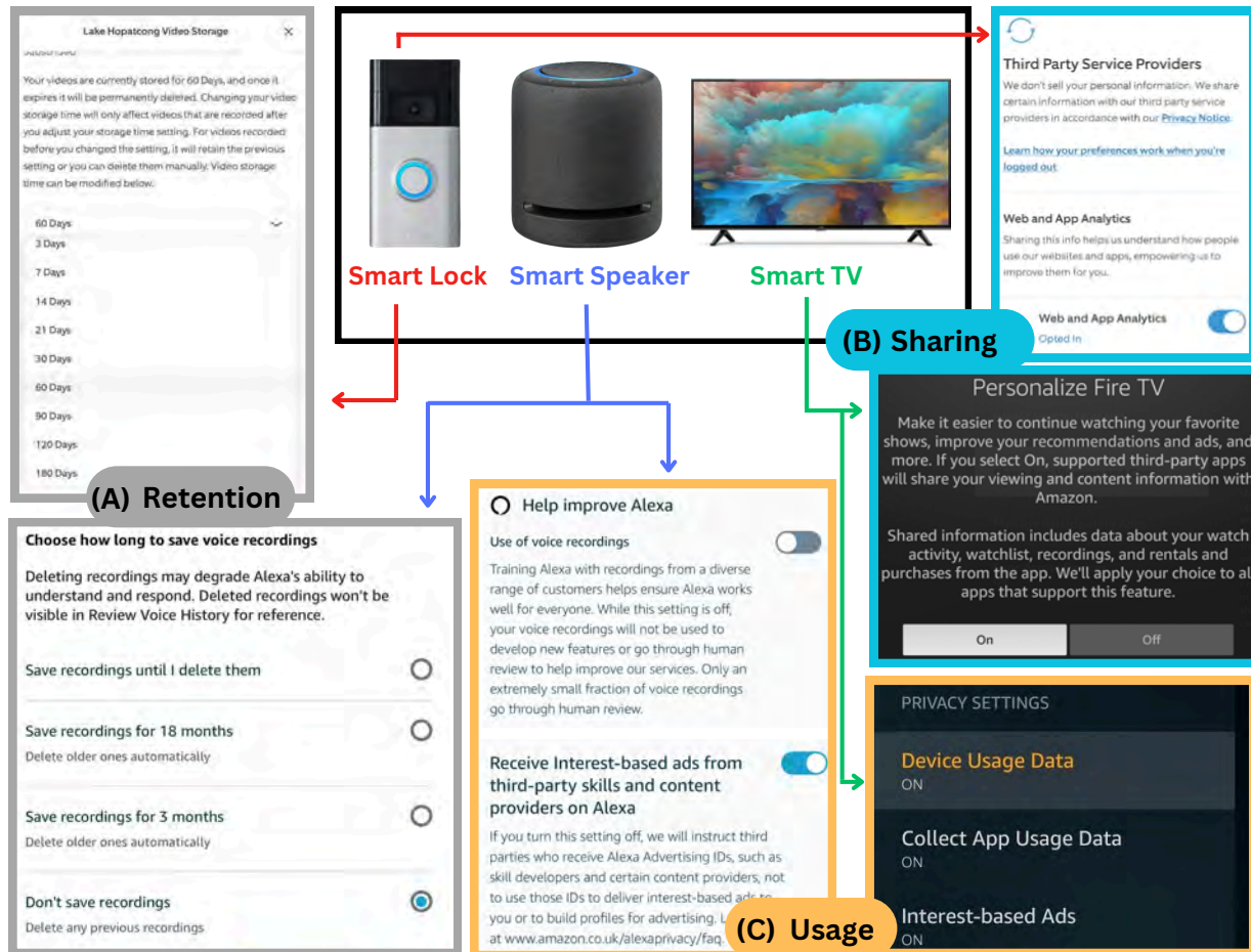
Figure 1: A composite representation of the varying menus and options available on three smart devices (Smart Lock [21], Smart Speaker [22], and Smart TV [23]) depicting each device’s privacy settings interface. (A) shows the privacy settings for retaining data, (B) shows the privacy settings for sharing data, and (C) shows the privacy settings for using data.
