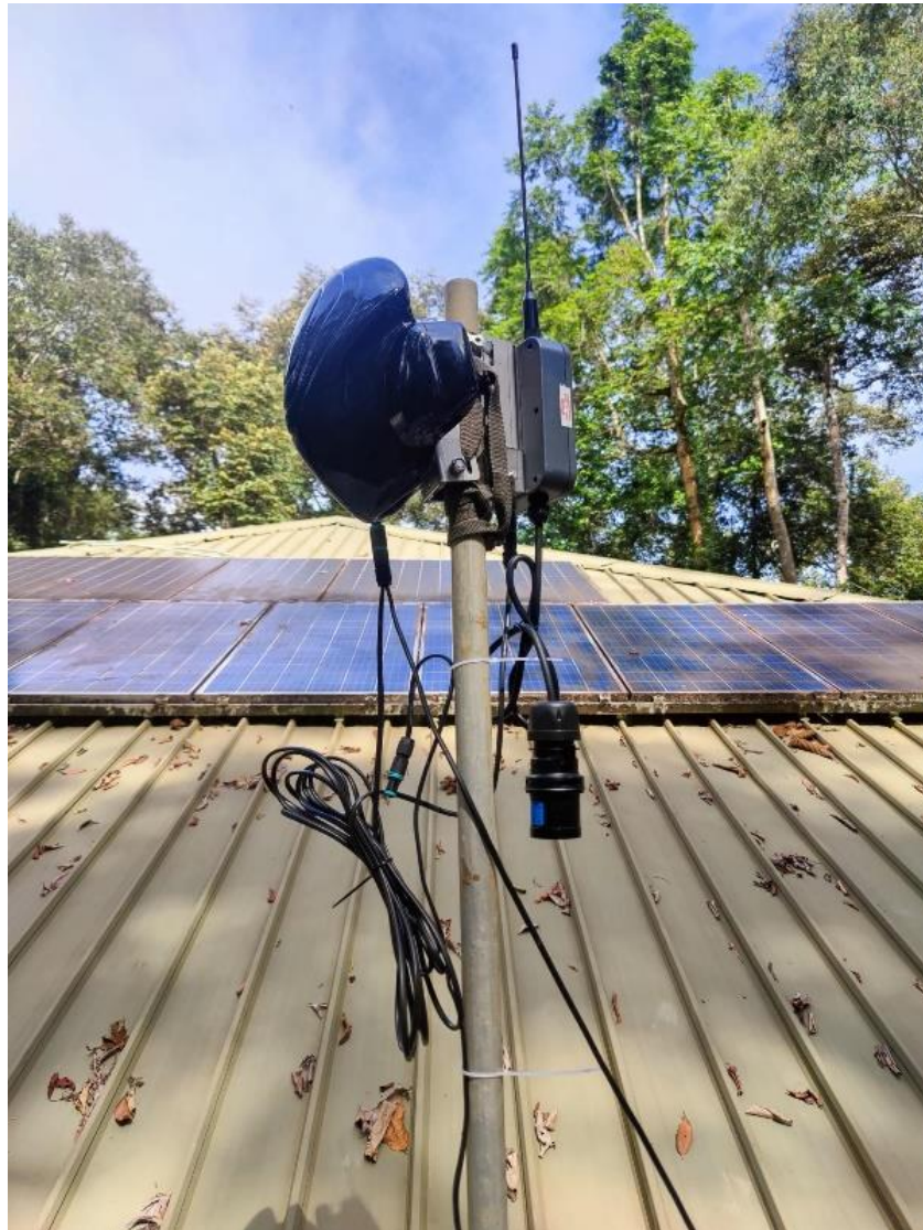
Figure 2.2. A closeup of Figure 2.1 showing the sensor and router installed on a pole.
