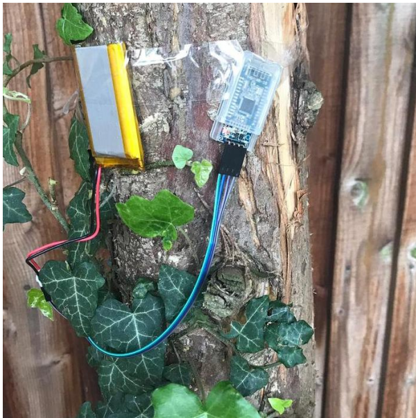
Fig. 2. HM-10 beacon mounted on a tree
