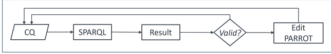
Figure 7: The validation process of the CQs begins with converting the natural language CQ into a SPARQL query, then running the query and checking the results. If the results are valid, the next CQ is run, and if not, the PARROT ontology is edited as appropriate.
