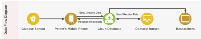
Figure 2: The DFD of Diabetes Treatment and Monitoring use case that was used to find the CQs by researchers.
