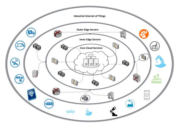
Fig. 2. Industrial IoTs and multilayer computing resources.
